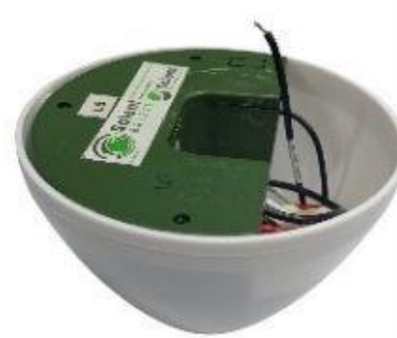
Position of 5 Speed Receiver Unit in LARGE Top Canopy
